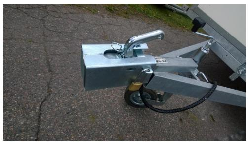
Picture 2. Attaching the trailer to the towing hitch
