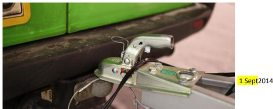
Picture 3. Trailer jockey wheel in the down position (trailer not attached to the vehicle)
