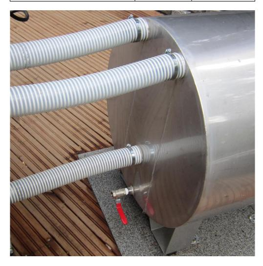
Make sure to open the water jacket tap of the stove after use. The tap is closed in this picture. The tap opens by moving the red handle laterally towards the tub.
